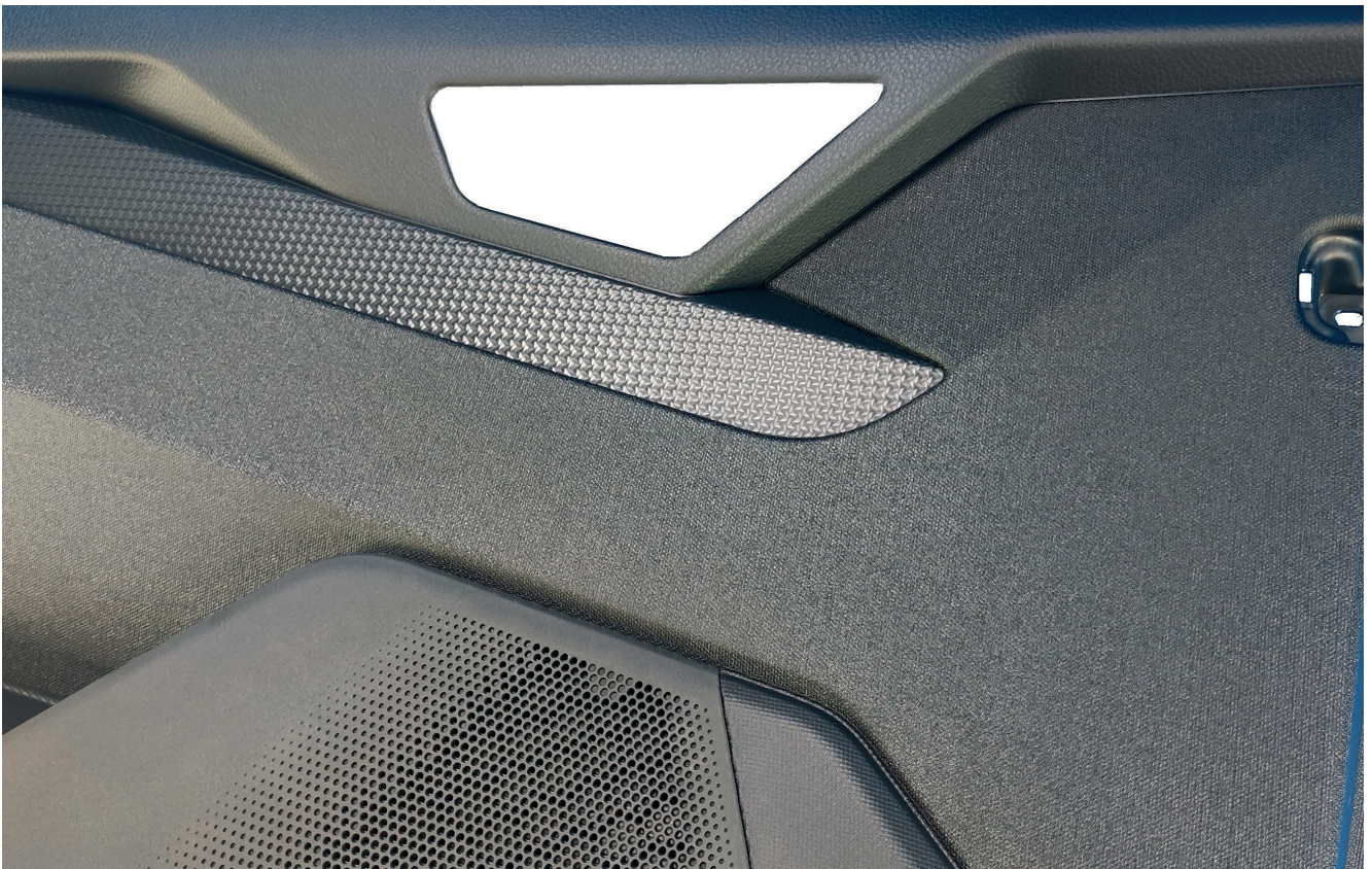
Single-source component: the door panel comes directly from the injection-molding machine as a ready-to-install visible component with different grains. © Faurecia
